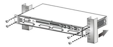
Figure 4-1 Install the NCT480 Box Chassis
